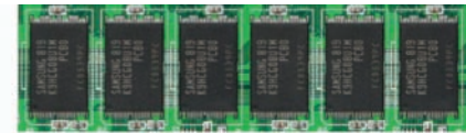
Solid State Drives use high-performance Flash Memory and have no moving parts
